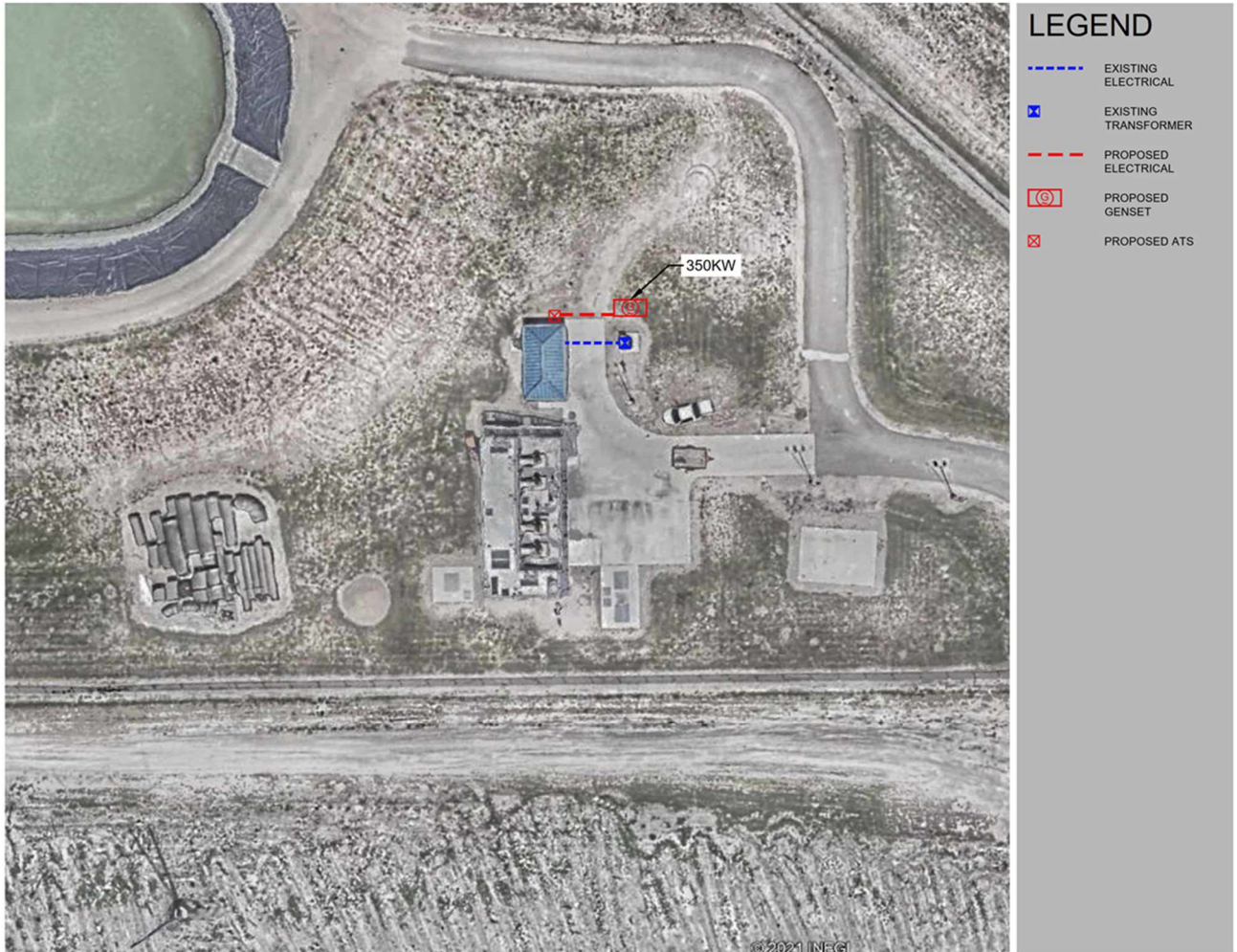
Figure 16: New Boeye Reservoir Pump Station Site Layout
