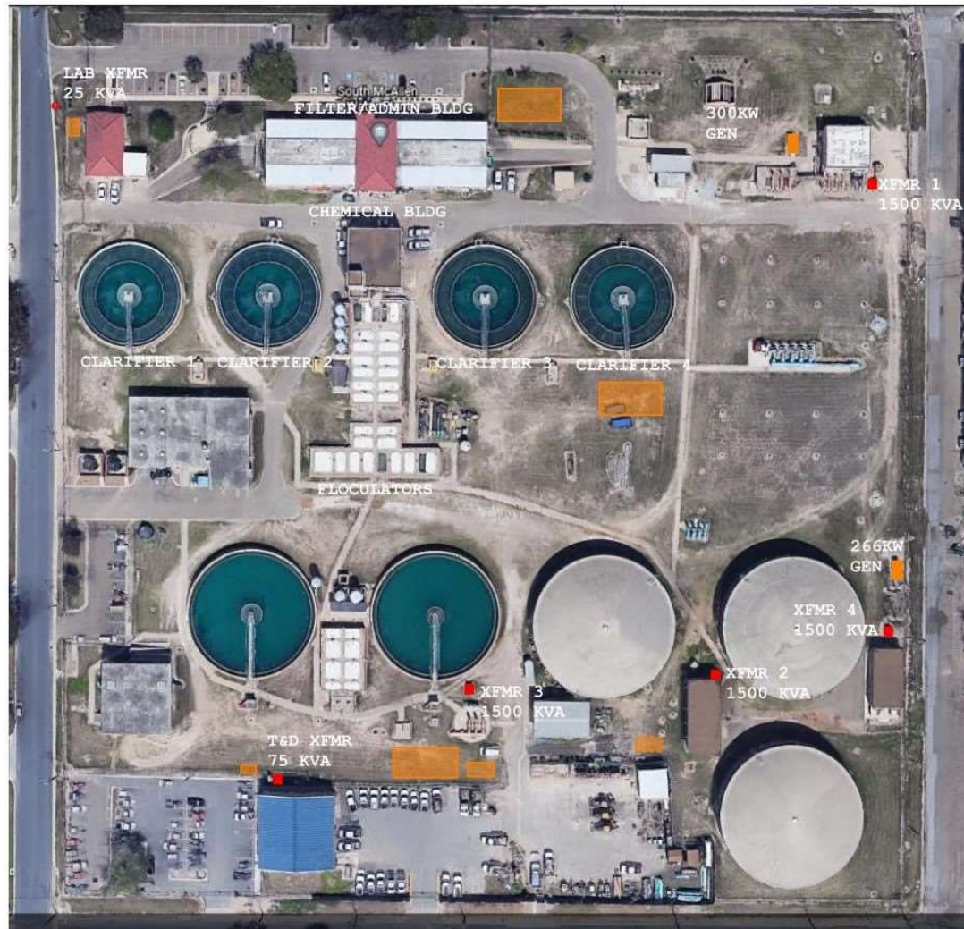
Figure 10: Possible Locations for New Generators
